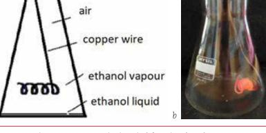
Figure 18: Copper wire in spiral form in ethanol vapours (a: preparation scheme and b: photo of the final reaction).
