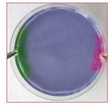
Figure 10. Colour change of the red cabbage juice during electrolysis with a bipolar electrode.
