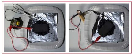
Figure 17: Aluminium/air battery with electric motor (left) or low-voltage LED lamp (right).
