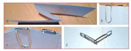
Figure 19. a-c : Folding the paper strip and attaching the paper clips. d: Connected paper clips after pulling up the paper strip.
