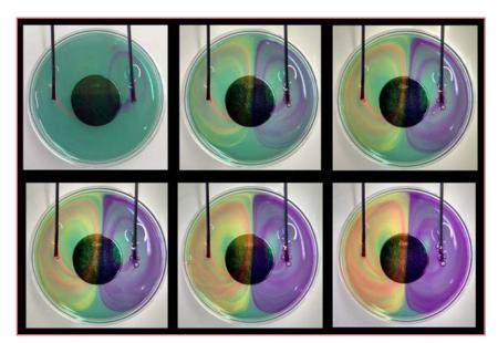
Figure 13. Development of water electrolysis with universal indicator in the magnetic field in 90s steps.
