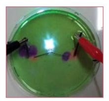
Figure 12. Electrolysis with an LED as bipolar electrode.
