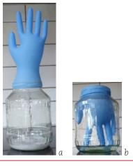
Figure 3. Expanding glove (a) against the air pressure and inverted glove (b) driven by the air pressure.
