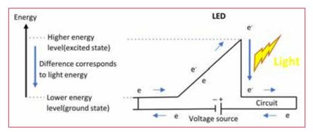
Figure 5. Simple model of an LED: A voltage source transports electrons to a higher energy level. From there they fall to a lower level, emit (light) energy and flow back in the circuit.
