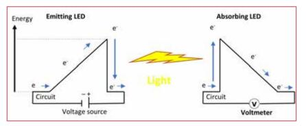
Figure 7. Model of energy transfer by quanta in the juxtaposition of an emitting and a receiving LED.
