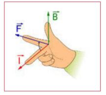
Figure 14. Right-hand rule for magnetic field, current and Lorentz force.
